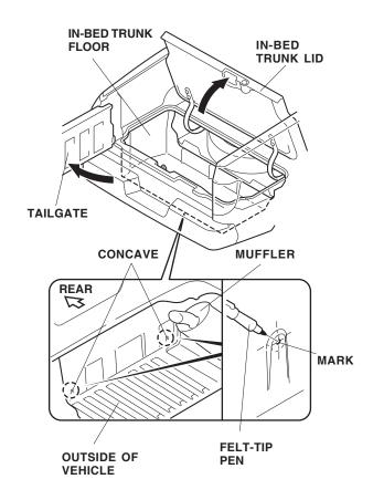
2. Under the rear of the vehicle, locate and mark the center of each concave on the outside of the trunk with a felt-tip pen.
